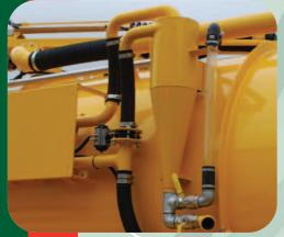
Hydro cyclone fitted to remove further debris particles from the recycled water.
