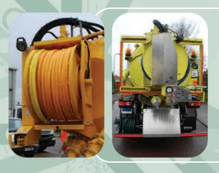
Main Reel Options available are 150 metres of 25mm on the Small Recycler and 150 metres of 32mm or 180 metres of 25mm on the Larger Recycler Machines. Also available is Traversing Reel option to shift the reel from side to side of the vehicle. Auxiliary Reel is 50 metres of 12mm fitted to the rear nearside of the vehicle.
