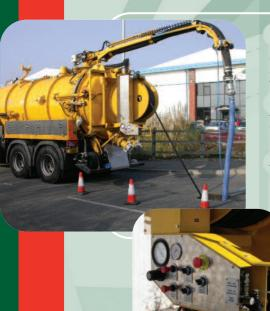
6" Pendant Operated Boom with Hydraulic Rotation extend and retract, Up and Down functions and Boom Valve Open and Close
