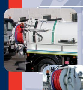
The Jet Vac Vehicle is equipped with Manual Handwheel catches with Hydraulic Door Opening and Hydraulic Tipping of the Tank .The Reel Pivots around the rear of the vehicle and is fitted with 100 metres of 19mm jetting hose with Operating Station at rear.The Rear Valves are both 4" Saunders with stack pipe on inlet with hose couplings to suit.
