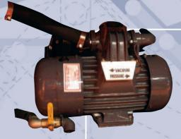
Vacuum Pump used is a Moro AC3 capable of 247 CFM with forced air cooling and builtin Oil Storage Tank with changeover valve and is fitted with Oil Catchment tank, Silencer and is hydraulically driven.
