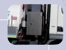
Hose Bins Option are open or closed bins either side Extra Storage Option is available giving a through storage area behind the cab and is fully lockable
