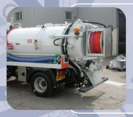
All Controls are situated at the rear once the PTO is engaged in the cab. Combination Units are fitted with interconnecting valve to enable use of the rear tank to carry water.
