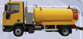
There are several types of this vehicle from a simple lightweight 800 gallon Sludge Tanker to Jetter Only Vehicles to the medium Volume 750 gallon Combination Jet Vac Tanker
