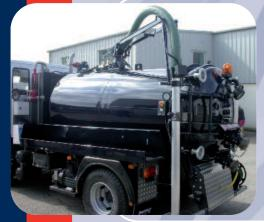
The 7.5 Tonne Range can also be equipped with a lightweight 4" Boom for Gully Cleaning work
